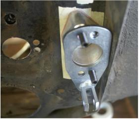
3.3 Cut-out the template created in step 3.1, inside the lines, and position over the outline on the firewall. Make sure the area inside the car is clear and drill two 21/64" holes.
