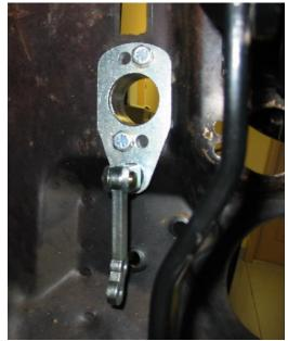
3.6 Remove master cylinder spacer block. Touch-up and deburr firewall as required.
